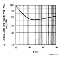
FIGURE 5. Noise Measurements
