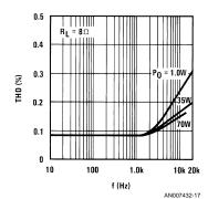
FIGURE 17. Distortion vs Frequency,  $R_L = 8\Omega$
