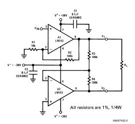
FIGURE 2. 130V Drive Across a Floating Load
