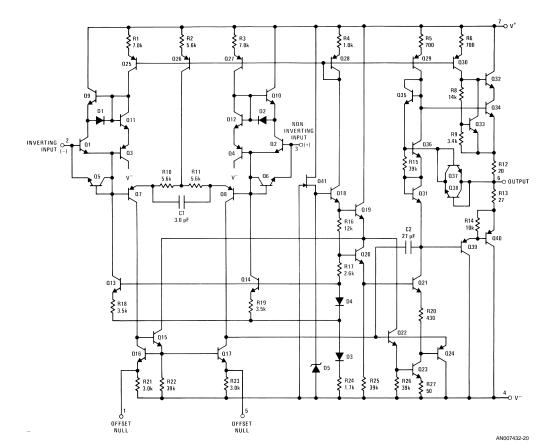
FIGURE 20. Complete Schematic of the LM143
