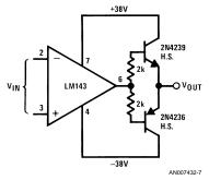
Heat sink is a Thermalloy No. 2230-5 or equivalent. All resistors are 10%, 1W.
