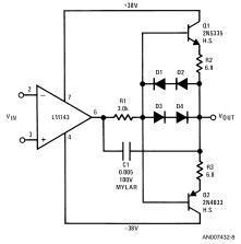
Heat sink is a Thermalloy No. 2230-5 or equivalent. All diodes are 1N914. All resistors are  $\frac{1}{2}$ W, 10%.
