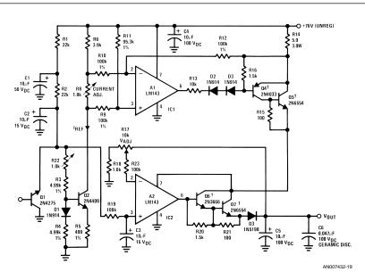
$\dagger Put$  on common heat sink, Thermalloy 6006B or equivalent. All resistors ½W, 10% unless otherwise noted. All capacitors 20%.
