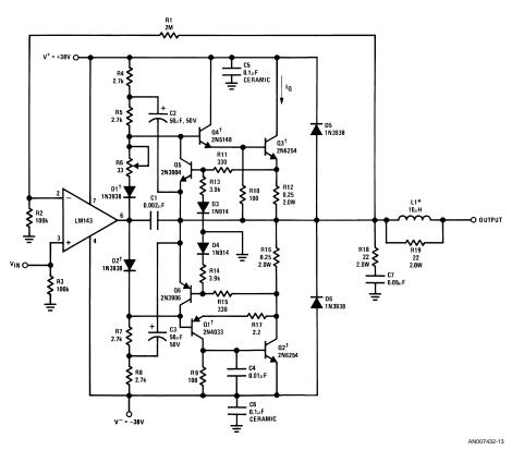
†Put on common heat sink, Thermalloy 6006B or equivalent.
