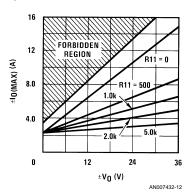
FIGURE 12. Maximum Output Current as a Function of R11 and V<sub>OUT</sub>
