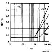
FIGURE 16. Distortion vs Frequency,  $R_L = 4\Omega$
