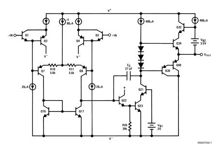
FIGURE 1. LM143 Simplified Schematic
