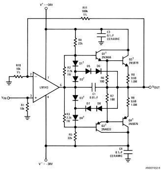
†Put on common heat sink, Thermalloy 6006B or equivalent.
