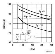
FIGURE 4. Common-Mode Rejection Measurements
