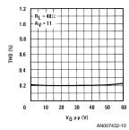
FIGURE 10. Harmonic Distortion Measurements
