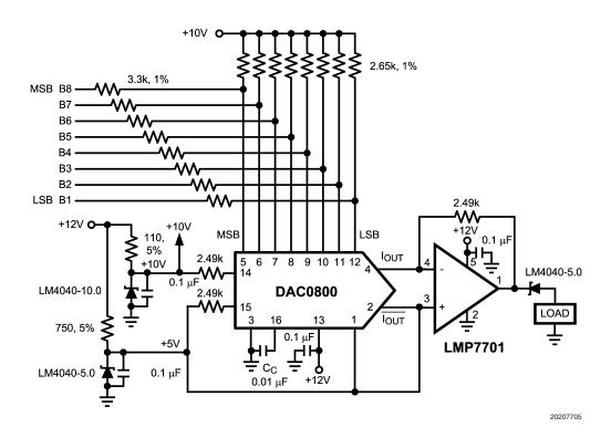
FIGURE 5. A complete single supply DAC0800 design with 0V to 5V output.
