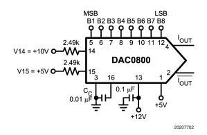
FIGURE 2. Positive only supply circuit for the **DAC0800**
