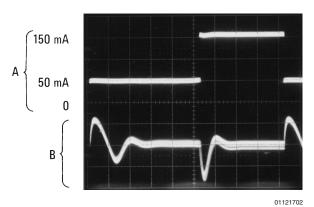
Load Transient Response A. Load Current, 50 mA/div B. Output Voltage Change 50 mV/div (AC-Coupled) Horizontal: 5 ms/div
