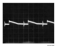
Output Ripple Voltage 20 mV/div (AC-Coupled) Horizontal: 5 ms/div
