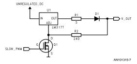
The LM3647 regulates the constant current source by turning the transistor Q1 on and off.
