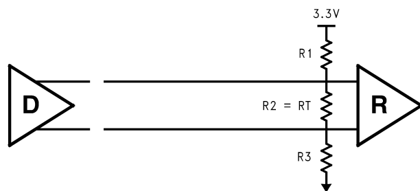
FIGURE 3. External Failsafe Biasing of an LVDS Link
