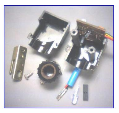
followed by the other half of the optical assembly. The assembly is then secured with the screws. The halves of the enclosure should fit closely together with little or no gap between them. The lens barrel should be able to rotate easily with a twist. It should not so loose that the tube rotates freely. The other mounting bracket should be attached at this time if one is used.
