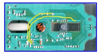
point for the sensor's data signal is an unused lead hole that must be cleared first. The wire attachment point for the sensor's clock signal is made by scraping away some of the solder mask off the indicated trace and lap soldering the wire to it.
