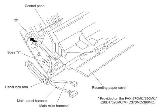
After securing the recording paper cover with the screws, be sure to route the main-panel
