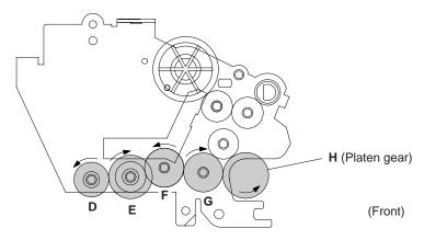
**Active Gears on the Scanner Frame ASSY**
