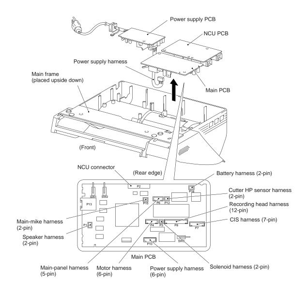
(2) Attempt to lift up the main PCB slightly. If it is impossible to lift up the PCB to an extent which allows you to disconnect the harnesses, you may not have unhooked the power supply harness core or cutter HP sensor harness core from bosses "C" or "D," respectively. Remove the ROM cover (refer to Section 1.2) and unhook those cores from bosses "C" and "D" illustrated below.
