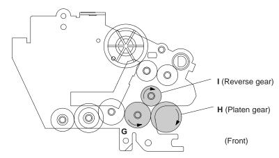
**Active Gears on the Scanner Frame ASSY**
