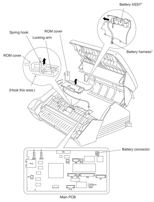
(FAX-270MC/290MC/520DT/520MC/ MFC370MC/390MC) (4) For the FAX-270MC/290MC/520DT/520MC/MFC370MC/390MC: To take out the main PCB or the power supply PCB in Section 1.18, unhook the battery harness core and cutter HP sensor harness core from bosses "C" and "D," respectively, at this stage.
