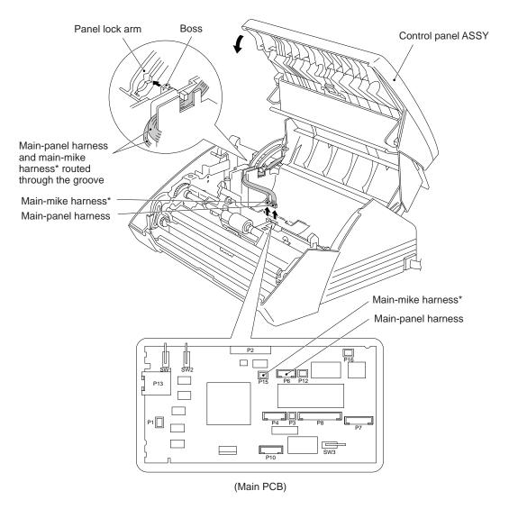
(FAX-270MC/290MC/520DT/520MC/ MFC370MC/390MC) (3) Push the control panel ASSY back and remove it.
