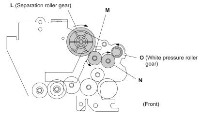
**Active Gears on the Scanner Frame ASSY**
