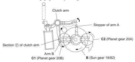
Arm B Blocked by Section ( of Clutch Arm
