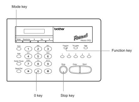
(4) To make the equipment return to the standby state, press the Stop key.
