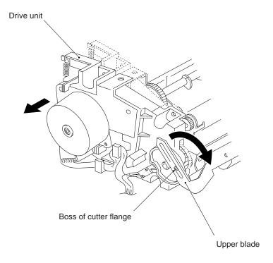
(7) To take out the motor, remove the screw, lightly press the locking arm and turn the motor counterclockwise. The motor bracket also comes off.
