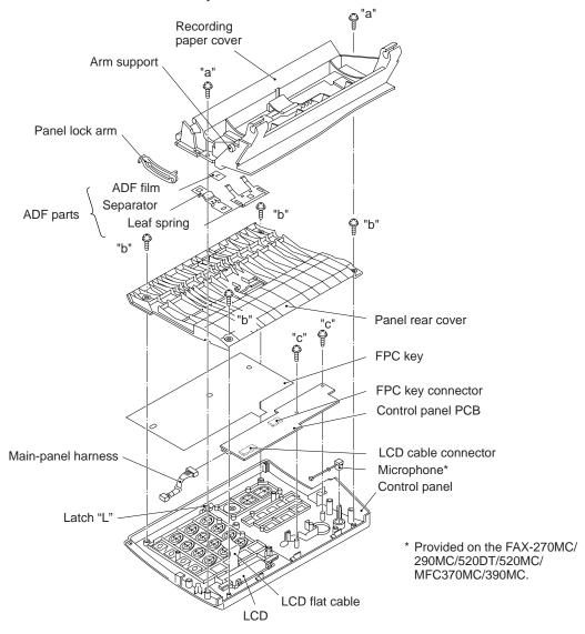
(8) For the FAX-270MC/290MC/520DT/520MC/MFC370MC/390MC: Take out the microphone\* and its harness\* from the control panel.
