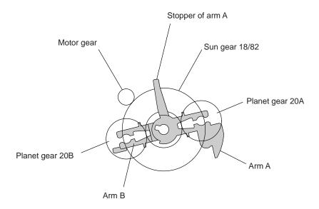
**Planetary Gear System**
