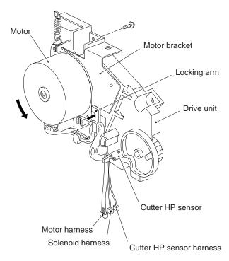
(8) To take out the cutter HP sensor, remove the screw.
