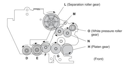
**Active Gears on the Scanner Frame ASSY**
