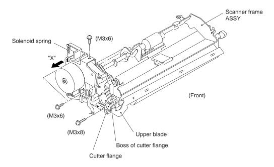
(6) After releasing the boss of the cutter flange from the upper blade, turn the upper blade clockwise as shown below and take the drive unit off from the scanner frame ASSY.
