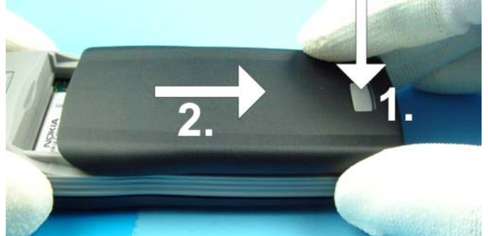
Press the Release Button before removing the Battery Cover.
