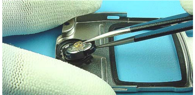
Use tweezers when removing the Speaker.
