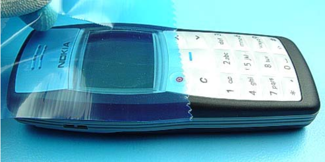
If not already done protect Window with a film to avoid dust and scratches.
