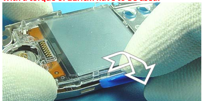
Unlock LCD snaps on both sides of the display.
