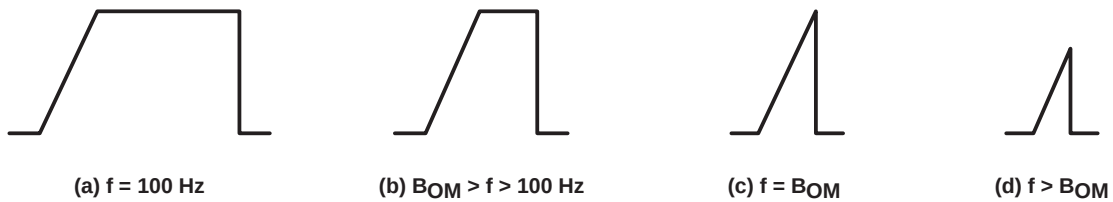
Figure 5. Full-Power-Response Output Signal
