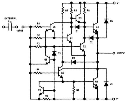
FIGURE A11-1. MH0025 Schematic (One-Half Circuit)
