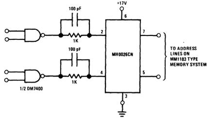
FIGURE A11-7. DC Coupled RAM Memory Address or Pre-charge Driver (Positive Supply Only)
