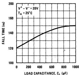
FIGURE AI-5. MH0025 Fall Time vs  $C_L$
