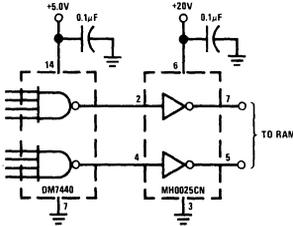
FIGURE A1-8. DC Coupled MH0025 Driving 1103 RAM.
